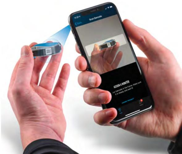
Center the serial number barcode for the device in the frame, and the team app will capture the device's identity and automatically assign it.
